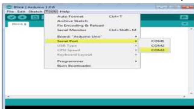
Ensure that the components in the Arduino IDE menu are working properly before sending the code to the board.
